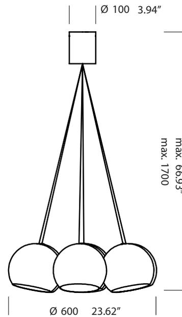
Installation note: Comes with a 4" backplate that mounts to a standard junction box
